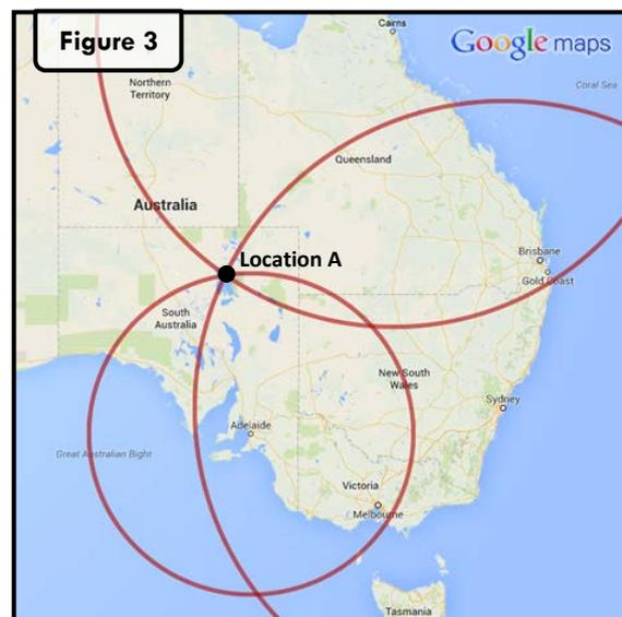
Trilateration also works in three-dimensions as well, but involves using spheres instead of circles and requires *four* distances to form a unique solution instead of three. GPS receivers use three-dimensional trilateration to tell you A) where you are on the earth and B) your current height.
