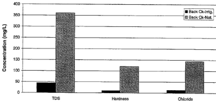
**Figure 2.25** A comparison of the average concentration of some ionic parameters in Back Creek during irrigation and natural flows in 1994 - '95.
