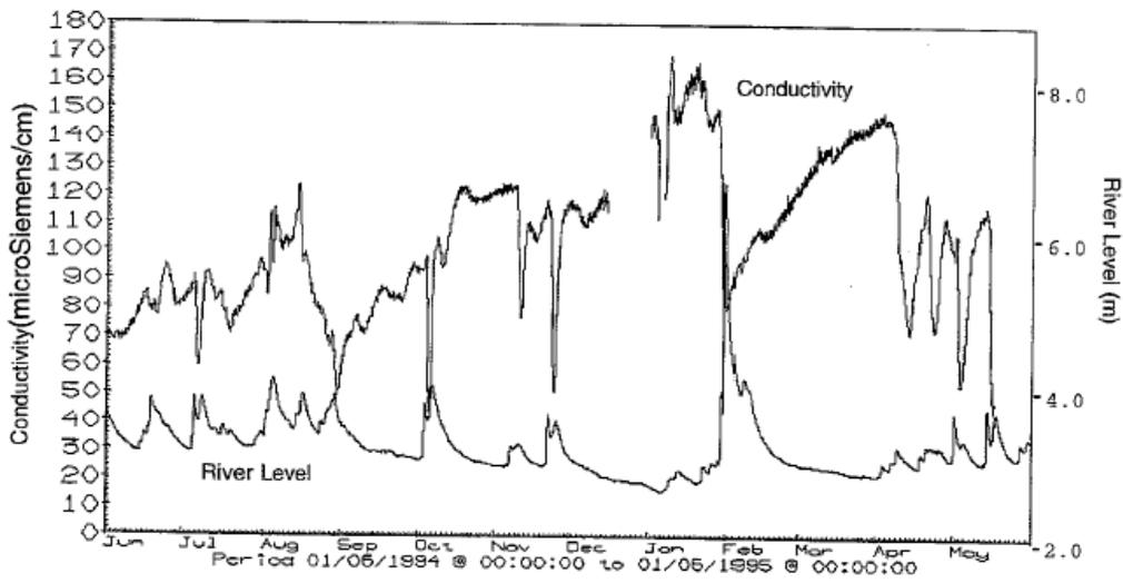
**Figure 2.8a** Time series of Conductivity and River Level for the South Esk at Perth between June 1994 and June 1995.
