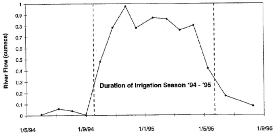
**Figure 2.22** Spot measurements of river flow in Back Creek during the 1994 - '94 irrigation season.
