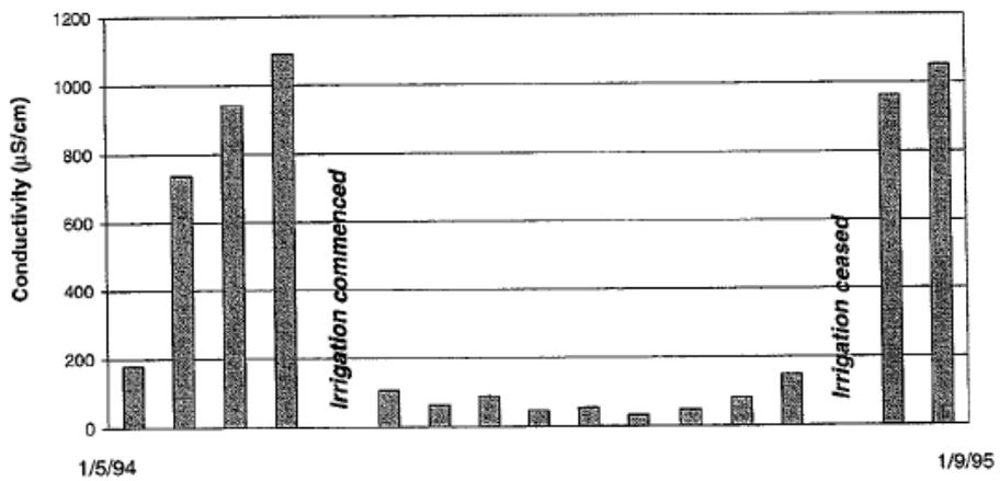
**Figure 2.23** Spot measurements of electrical conductivity in Back Creek during the 1994 - '94 irrigation season.
