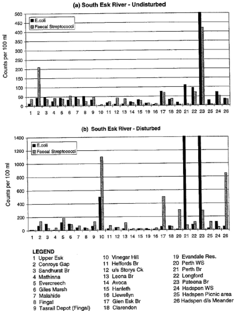
**Figure 2.28** Longitudinal transect of the South Esk River, sampling undisturbed flowing water (a) and sediment disturbed water (b) for faecal coliforms and faecal streptococci. Survey carried out in late November, 1994.
