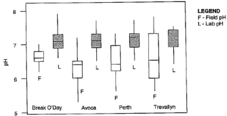
**Figure 2.10** Comparison of field read pH and lab determined pH for four sites in the South Esk catchment.
