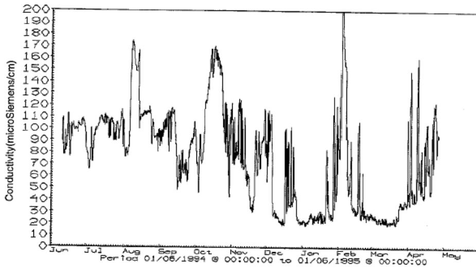
**Figure 2.8b** Time series of Conductivity for the South Esk at Longford between June 1994 and June 1995.
