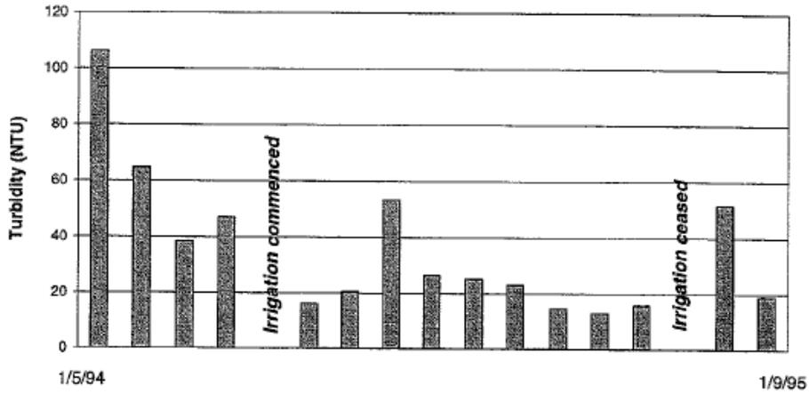
**Figure 2.24** Spot measurements of turbidity in Back Creek during the 1994 - '94 irrigation season.
