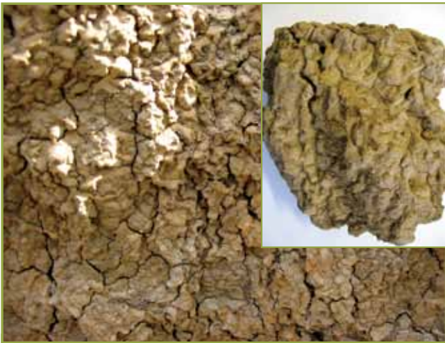
Figure 2 (a). Example of dribble pattern on an exposed subsoil, the photograph was taken from within an actively eroding tunnel system. (b) Dribble patterns on sodic soil ped.
