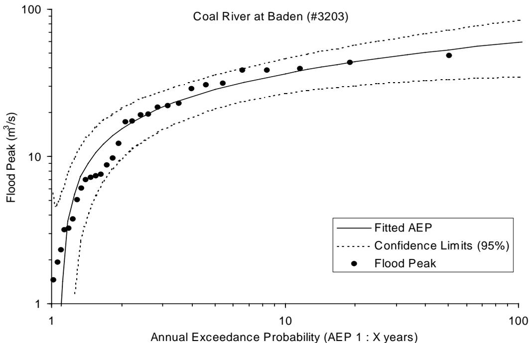
**Figure 6.1** Flood frequency curve for Coal River at Baden.
