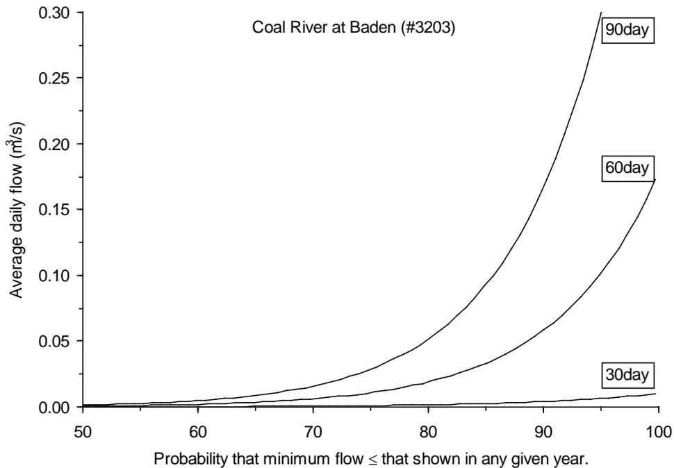
**Figure 5.2** Low flow frequency curves for Coal River at Baden.
