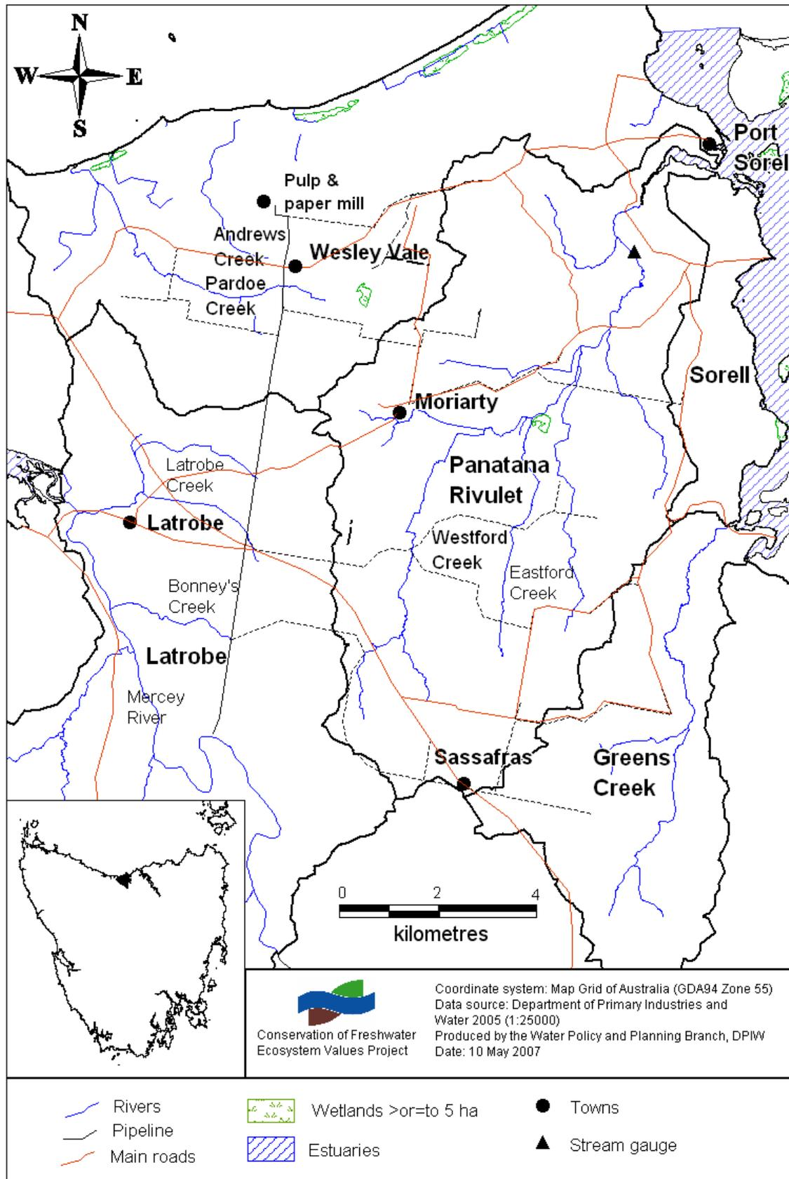
**Figure 1.** Surface water drainage in the SassafRAS – Wesley Vale area including the stream gauging station and subcatchment areas. CFEV, © State of Tasmania and the LIST.
