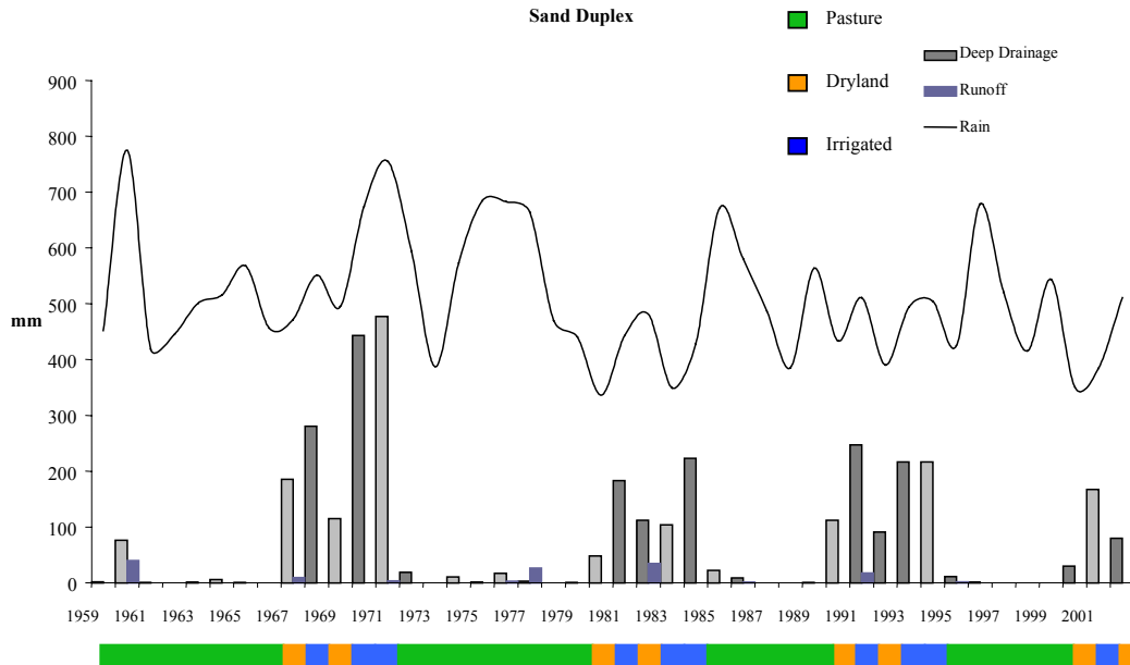
Figure 11. 44 years of modelled deep drainage and runoff under crop rotations on a sand duplex.
