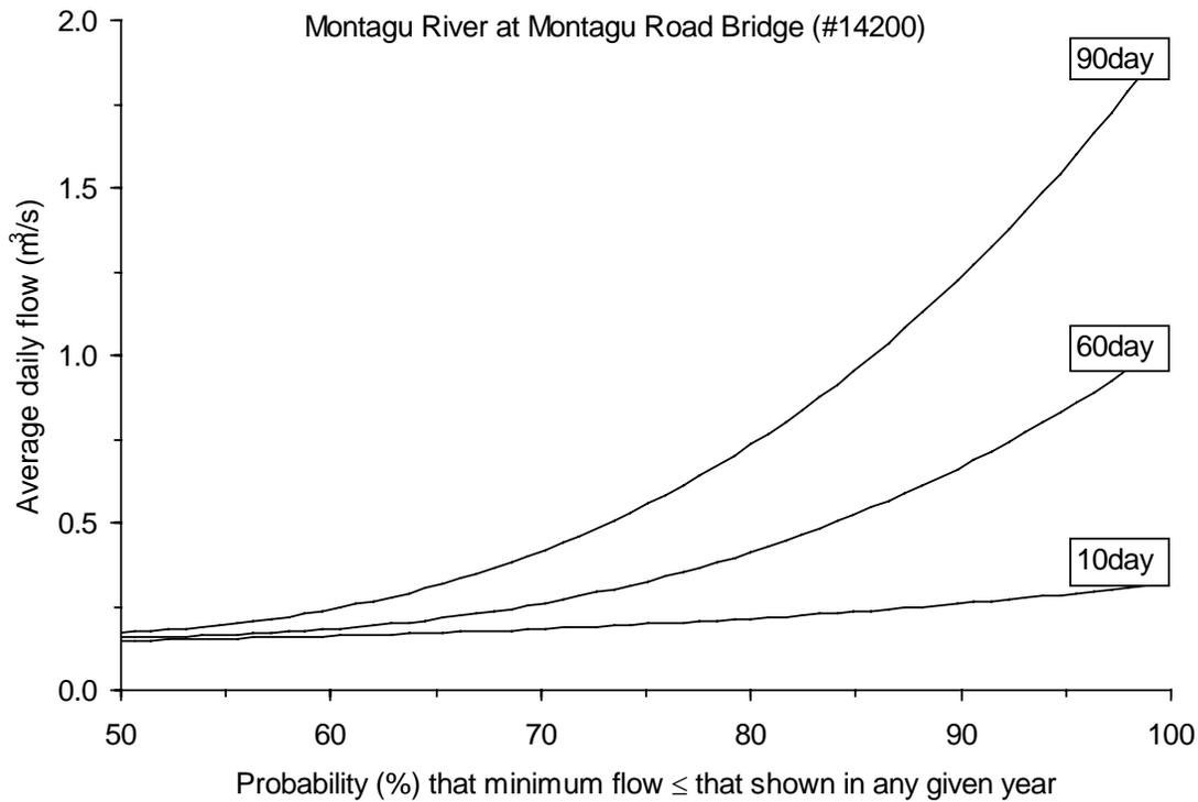
**Figure 5.2** Low flow frequency curves for Montagu River gauging site.
