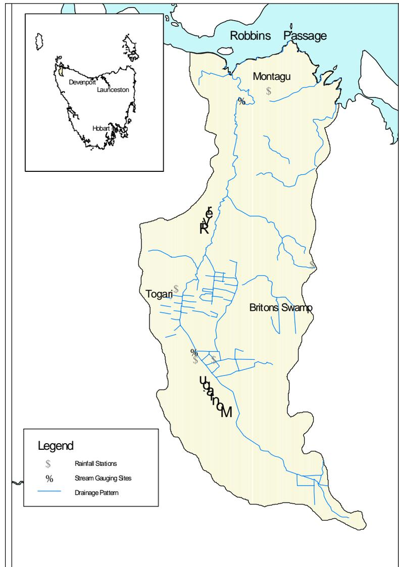
**Figure 1.1** Hydrological set up of Montagu River catchment.
