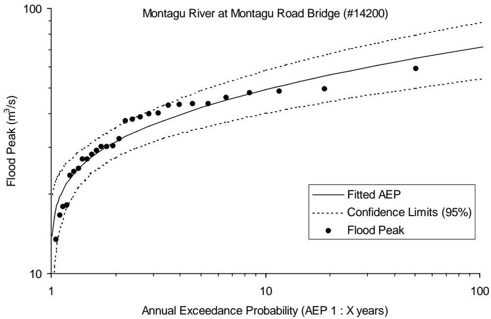
**Figure 6.1** Flood frequency curves for Montagu River gauging site.
