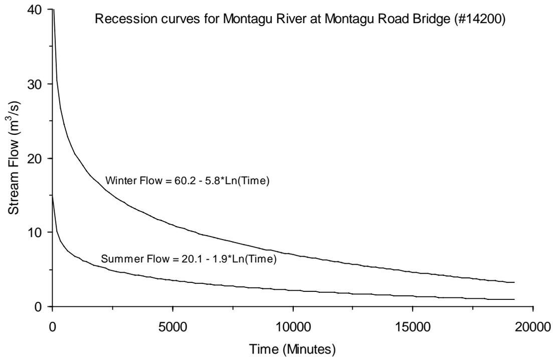
**Figure 5.1** Recession curves for Montagu River at Montagu Road Bridge.
