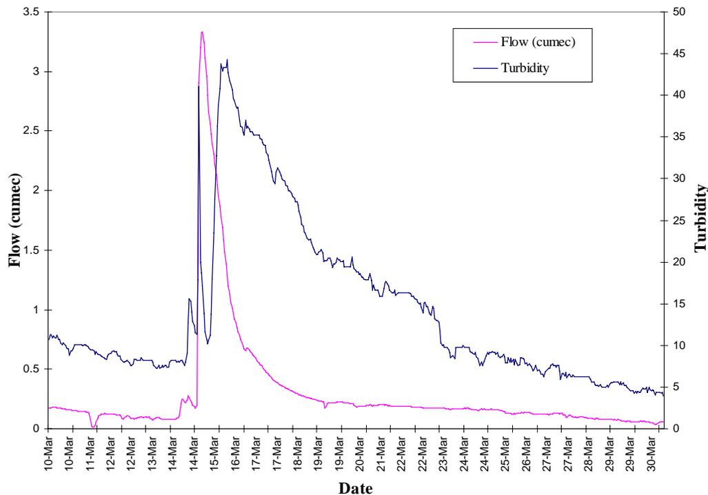
**Figure 3.3:** Graph of discharge and turbidity collected from CR3 (Coal River at Richmond) during a flood event that occurred between 14<sup>th</sup> and 30<sup>th</sup> of March 1999.
