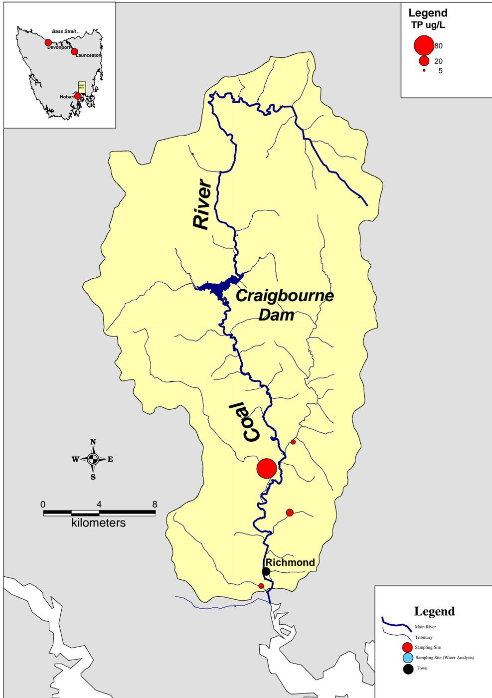
**Figure 2.42:** Survey of total phosphorous concentrations recorded in the Coal catchment on the 18<sup>th</sup> July.
